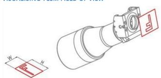
Field of View with detector's long side set horizontal
