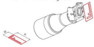
Field of View with detector's long side set vertical
